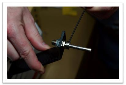
9) Slide the wheel onto the axle and secure with cotter pin. NOTE: The wheel hub thickness has changed and may require an additional 7/32" wheel collar between or in place of cotter pin and the wheel.
