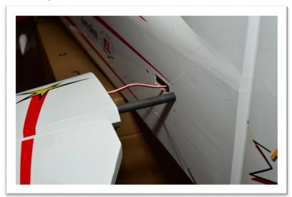
24) Secure the stabs with the provided bolts and washers. Be sure to check these bolts after every flight!
