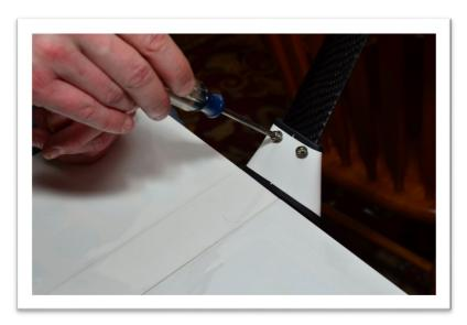
8) Install the landing gear axles through the hole on each side in the landing gear with the provided nylon lock nuts. Place a wheel collar onto the axle about 1/4" from the base and secure the grub screw.
