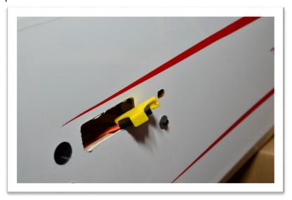
22) Tie the provided string in the tail to your 2x 48" servo extensions and pull them through the fuselage tube.
