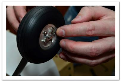
10) Secure the wheel pants with the small hex bolts, washers and some Loctite.
