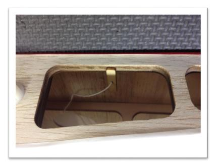
23) Slide in the small carbon fiber tube into the tail and connect the servos to their extensions. Always use a servo keeper on these! Slide each elevator half onto the tube, tucking the extra servo wire into the fuse.
