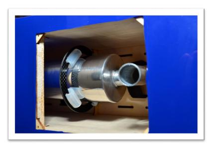
29) You can now re-mount your engine, mufflers and ignition box. The ignition box can be placed anywhere, but typically goes on the top or side of the motor box. In our example, it's been mounted to the firebox access hatch on the top of the motor box. Don't forget to locktite everything!
