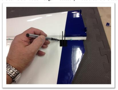
15) Remove the assembly and use a sharp blade to cut approx. 1/16" in from your line and remove the covering. Use caution to only cut deep enough to remove the covering and not cut into the balsa! A hot blade can help here. Remove your lines with a paper towel soaked with denatured alcohol.
