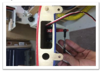
21) If necessary, cut open the holes in the tail of the fuselage for the tail tube, servo exits, and anti rotation pins.
