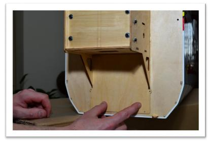
33) Cut the cowl as needed to clear the mufflers as well as extra for exiting air. No cuts should be required to clear the DA-70 heads and spark plugs. Add baffling with balsa or craft foam as desired to direct airflow over the engine heads and out the exit in order to keep your engine running cool & happy. Baffling is not required, but is always a good idea.
