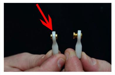
14) Test fit the control horns into their slots in each elevator half to make sure they will fully seat down. Sand the corners or bottom edge if necessary. Trace around the base plate with a fine Sharpie.
