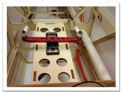
51. Slide an aluminum crimp tube onto the end of one of the wires, and then loop the wire through the pull-pull fitting, through the crimp tube the other way, and then loop it into the crimp tube a second time. Crimp at least twice with a crimper tool or side cutters. Be careful not to actually cut the tube or wire by using too much force with side cutters!
