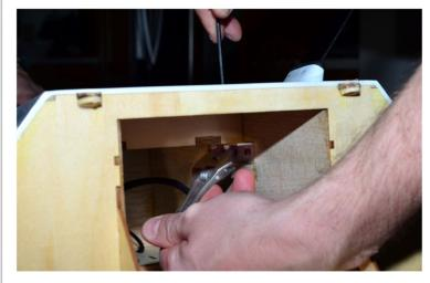
6) Place the wood filler block over the landing gear. Pay attention to the fit as it is directional. While the cuffs will hold this in place, we suggest using a piece of clear tape, or white Ultracote for extra security.
