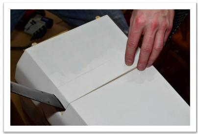
7) Install the landing gear cuffs using the 4 phillips head bolts and washers provided. You may alternatively use silicone glue. If the cuffs don't match well to the fuselage, remove and carefully heat & mold them with a heat gun.
