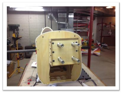
35) Mount the motor to the standoffs using the hardware provided by the motors' manufacturer. Don't forget to use blue locktite on all bolts!
